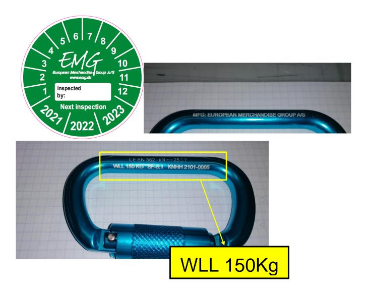
WLL (Working load limit) is defined as the maximum load that must be applied on the lifting equipment.
