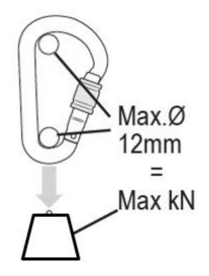
Make sure it is locked before lifting. Lifting is not allowed before the device is locked.
